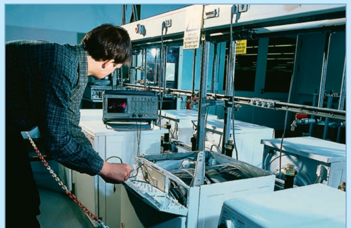
Series-accompanying lifespan and reliability tests of electronic components for tumble-dryers
