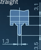
PCB terminal 1,3x0,5 mm straight
