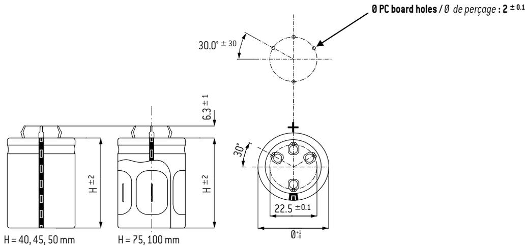
Dummy pins near positive terminal are for mechanical support only.
