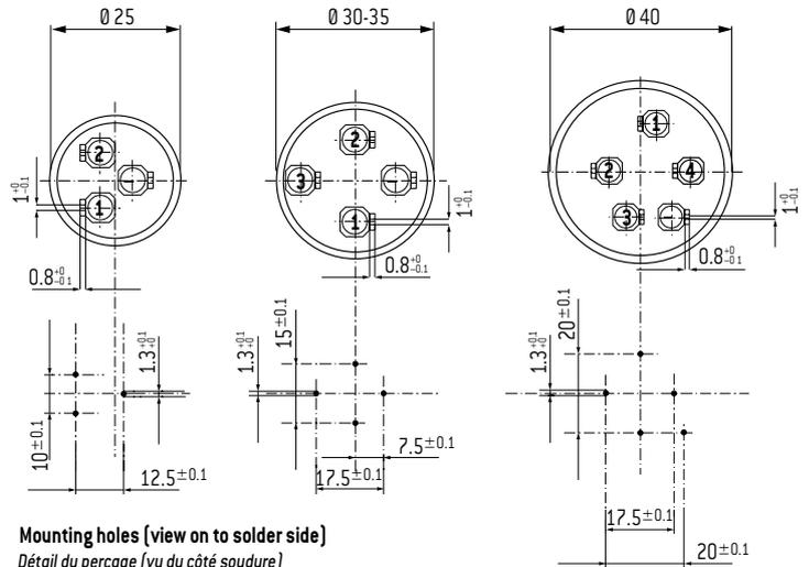
Mounting holes (view on to solder side)
