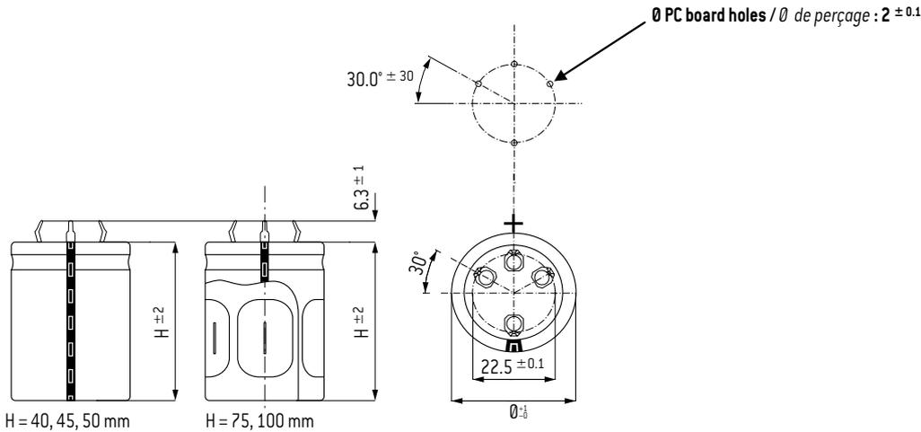
Dummy pins near positive terminal are for mechanical support only. They must be electrically insulated from the positive and the negative terminals.
